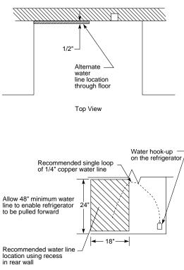
Installation of Water and Electrical Outlets
