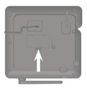
2. Place the battery in the compartment. Make sure the supplied battery with the label **THIS SIDE UP** faces up, as indicated.
