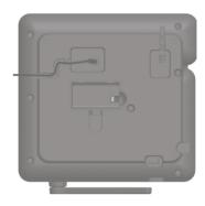
3. Align the cover flat against the battery compartment, then press down until it clicks into place.
