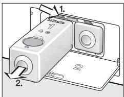
Press the yellow release button (1.) and pull the container out (2.).
