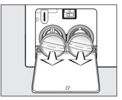
Remove the drain filters completely.
