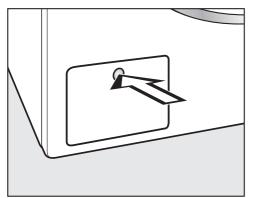
Press the drain pump access panel.
