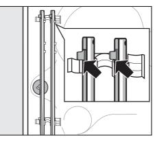
Secure the transit bars to the back of the washing machine. Make sure the top catch is located above the holder.
