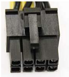
8-pin (4x2) PCI-E Connector
