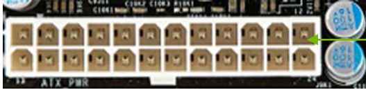
Figure 4. PWR1 Motherboard Connector
