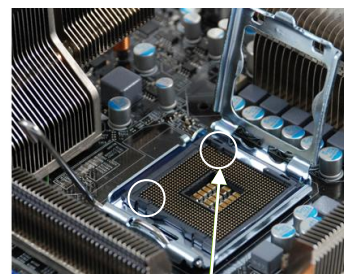
Align notches with notches on the CPU
