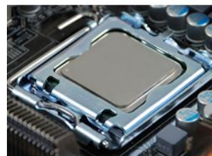
Align notches with notches on the CPU
