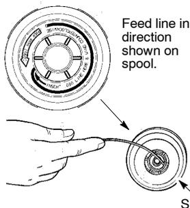
2. Insert one end of line into center cavity of empty spool. Ensure line will feed into spool in the direction shown on the spool (counterclockwise).
