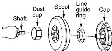
Use a pre-wound spool or refill spool with line. If using a pre-wound spool, remove tape strip from line and spool.
