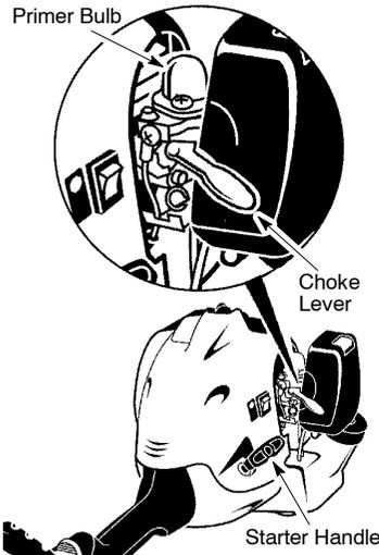
5. Pull starter rope handle sharply until engine sounds as if it is trying to start, but do not pull rope more than 6 times.
