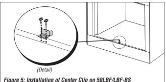
Figure 5: Installation of Center Clip on 50LBF/LBF-BS
