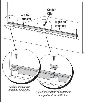
Figure 3: Installation of Air Deflectors and Center Clip on 36LBF/LBF-BS and 42LBF/LBF-BS
