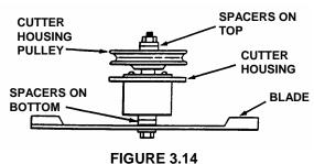
**NOTE**: Changing the cutting height of Blades DOES NOT change the Deck ground clearance. If an undesirable cutting pattern results, then cutting height adjustment MUST be made by adjusting Mower Deck height and Caster Wheels.
