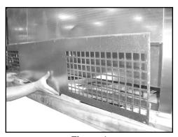
Figure 1 "Removal of Rear Grill"
