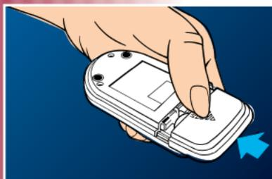
1. Press firmly on "open" arrow and slide forward in the direction of the arrow. The lid releases.
