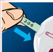
2. With the Meter off, hold the round end and insert the Test Strip fully into the Meter. You will hear a beep.
