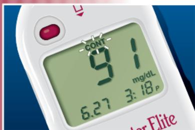
**Mark the Result:** Hold the button until "CONT" appears at the top of the display. Release the button and "CONT" begins flashing. Remove the Test Strip while "CONT" is flashing.
