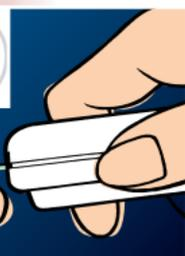
4. Touch and hold the TEST END (tip) of the Test Strip to the drop of blood until the Meter beeps. The Test Strip is filled, and the timer begins counting down from 29 seconds.
