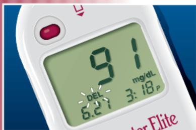
**Delete the Result:** Hold the button until "CONT" appears at the top of the display. Release the button and "CONT" begins flashing. Push the button again, "DEL" begins flashing above the date. Remove the Test Strip while "DEL" is flashing.
