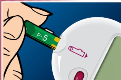
2. Insert the Code Strip into the test slot as shown. A beep sounds and a full display appears briefly. Another beep sounds and the Code Number (for example F-5) appears in the display.
