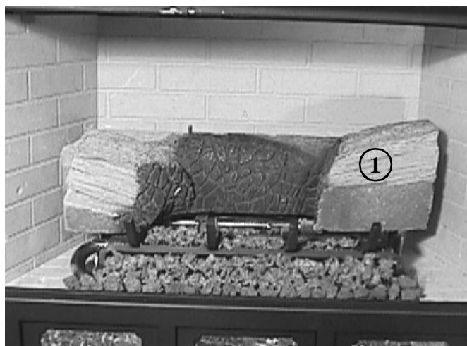
Locate two holes in bottom of rear log. Place the rear log down over the two pins to locate the log.
