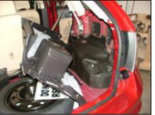
**STEP 7** Remove passenger side cargo panel by prying away from side of vehicle and floor.
