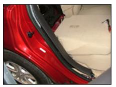
**STEP 6** Pull passenger side cargo panel away from the door jamb.
