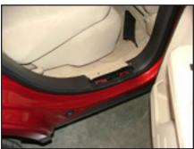
**STEP 5** Remove passenger side threshold plate.
