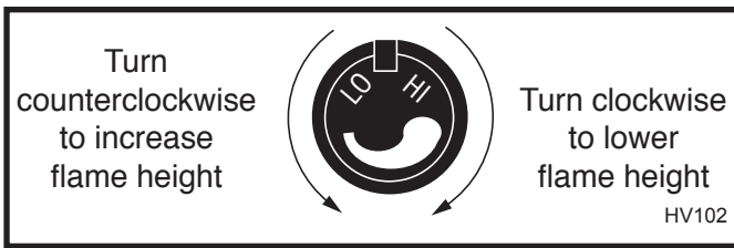
Fig. 18 Flame adjustment on gas valve.
