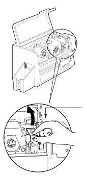
**2.** Open Printer cover and locate Cleaning Cartridge place. Remove the yellow adhesive.
