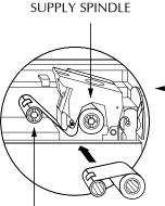
**3.** Load ribbon onto the supply spindle (under print head carriage) and empty core (with tape attached) onto the takeup spindle. Make sure the ribbon comes off the top of the supply spindle and feeds to the top of the take-up spindle.
