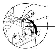
Open Cover, and adjust lever to correct position. Repeat for different card thickness. (Factory setting is for 30mil (0.762 mm) card thickness. See diagram below :
