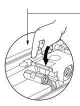
**4.** Push down on the Print Head Lock Lever until an audible 'click' signals the locked-down position.
