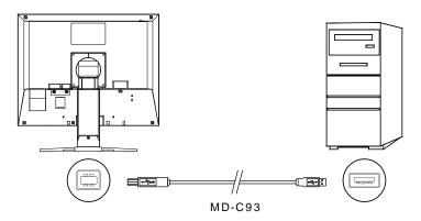
2 Connect the measurement device to downstream port of computer; USB keyboard or the monitor:
