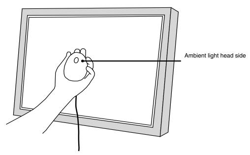
After the measurement, click [OK]. The measured value is set as the target white of the configuration window.
