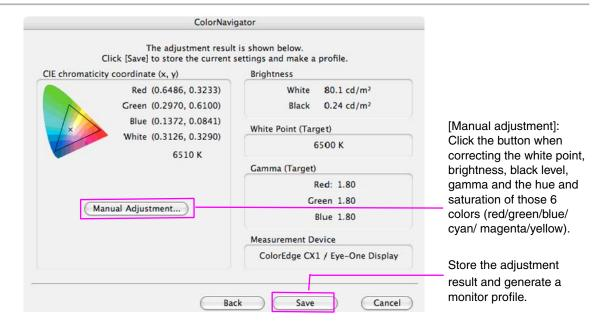
• If the black level is shown as minus value, start calibration from the beginning again. Light could have seeped through to the sensor of the measurement device during initialization. Be sure to attach the measurement device to the monitor closely.
