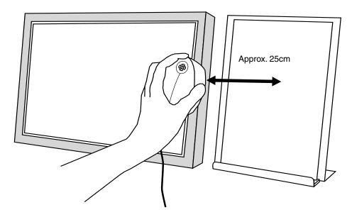
After the measurement, click [OK]. The measured value is set as the target brightness and white of the configuration window.
