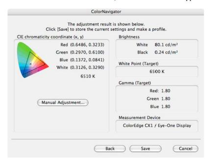
• If the black level is shown as minus value, start emulation from the beginning again. Light could have seeped through to the sensor of the measurement device during initialization. Be sure to attach the measurement device to the monitor closely.
