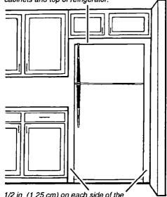
1/2 in. (1.25 cm) on each side of the refrigerator for easier installation.
