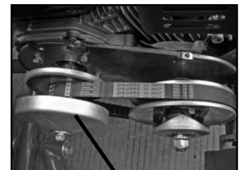
4. Install drive cover and weight assembly. Make sure bolt on driven and nut on driver are snug.
