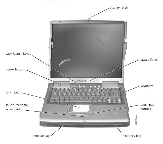
**DISPLAY LATCH** — Keeps the display closed.
