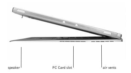
**SPEAKER** — Use the volume wheel or press the volume control keyboard shortcuts to adjust the volume of the integrated speakers. For more information, see the **Tell Me How** help file. To access the help file, see page 17.
