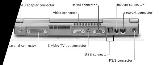
**AC ADAPTER CONNECTOR** — Attach the AC adapter to the computer.
