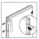
Fix the handle on the opposite side, insert the plastic plugs into the holes left open that can be found in the instruction for use bag. Reposition, level the appliance, wait for at least two hours and then connect it to the power socket.
