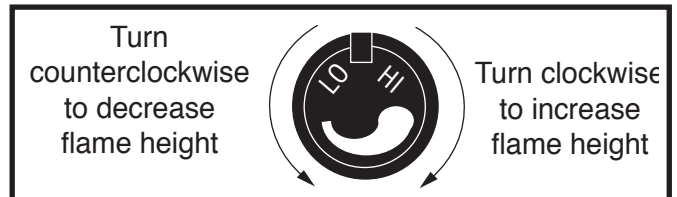
Fig. 23 Flame adjustment knob for Honeywell valve.
