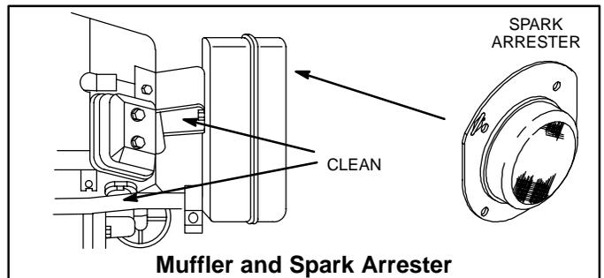
**Muffler and Spark Arrester**
