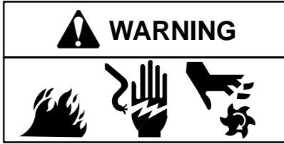
If you perform any maintenance on the engine, first disconnect the spark plug wires from the spark plugs, and disconnect the battery at the negative terminal (electric starter engines only) to prevent unintentional sparking. Unintentional sparking can result in fire or electric shock. Unintentional start-up can result in entanglement, traumatic amputation or laceration. Use only correct tools.
