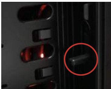
Lock lever in default, unlocked position.
