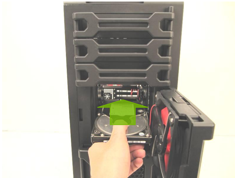
Installing a 3.5" internal device
