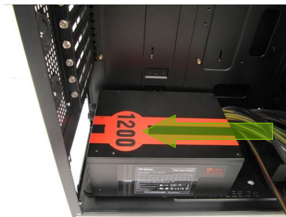
PSU resting on the standard ATX PSU mount.
