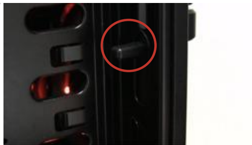
Slide the lever to its most upward point to lock access doors.
