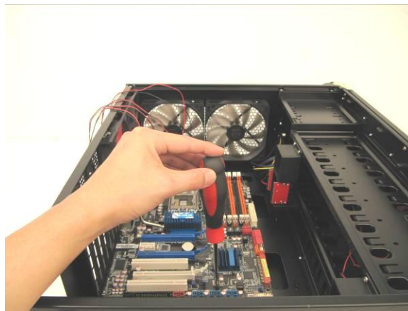
Step 5: Screwing in the motherboard after standoffs are installed
