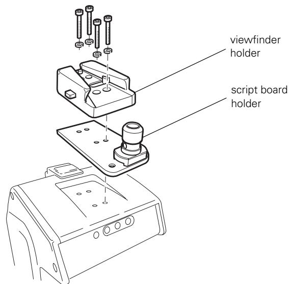
4. The script board can now be mounted onto the bracket.
