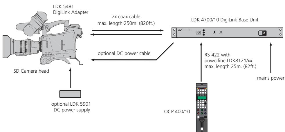
When a DC power cable is used to power the camera from the base unit, refer to section 6 for the pin layout of the DC connectors. The maximum length of the cable depends on the type of cable and the power used by the camera. The table below is an indication of the cable lengths that can be used.
