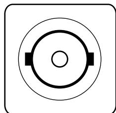
Apply a 1Vpp, 75 Ohm video signal to this BNC socket for viewing in the camera viewfinder (or via the VF/CVBS BNC output socket).
