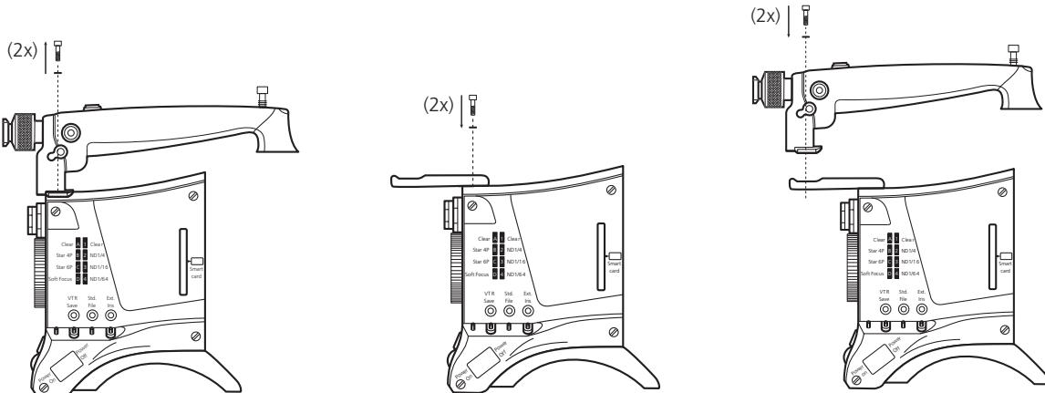
5. For LDK 500: fold the flat cable away into the hollow part of the carrying handle.
