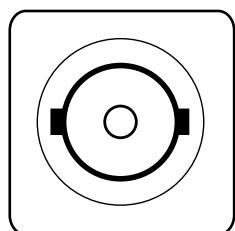
This BNC connector supplies an SDI video output signal (Y/Cr/Cb 4:2:2) that also includes embedded audio, intercom and private data signals.
