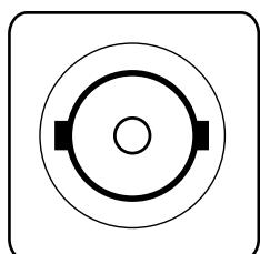
Apply a 1Vpp, 75 Ohm genlock signal- (C)VBS or Black Burst) - to this BNC socket to synchronize the camera.
