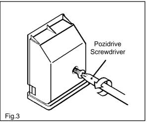
Prise cover loose using screwdriver in position
