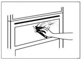
DO NOT ATTEMPT TO REMOVE ANY OF THE CONTROL KNOBS FROM THE PANEL AS THIS MAY CAUSE DAMAGE AND IS A SAFETY HAZARD.
