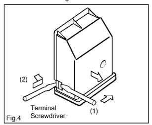
Lift cover and remove screw from cable clamp.
