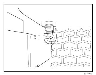
Fuel shut off valve in OFF position
