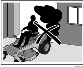
Never drive the machine in an enclosed space
