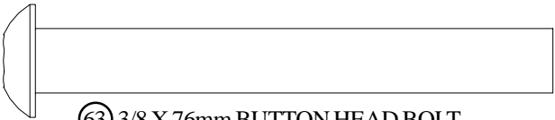
63 3/8 X 76mm BUTTON HEAD BOLT
