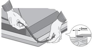
• Do not fix the hob using silicon as this would make it impossible to uninstall the hob, if necessary, without damaging it.
