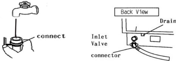
6. If leaks are located, immediately shut the water supply and check the hose connections fully. Tighten connections if necessary.
