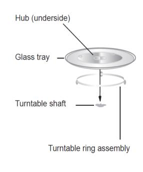
> Before first use, check that any securing tape has been removed from the glass tray and turntable ring assembly. These parts must never be restricted from rotating.
