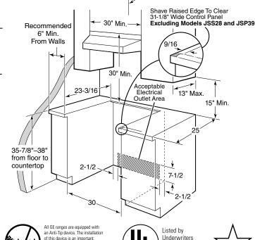
of this device is an important. required step in the installation
