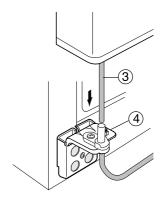
3) Insert the upper hinge shaft (⑤) into the hole (⑥). After levelling between the upper hinge hole (⑦) and the hole of the cabinet (⑧). Reattach hinge screws (⑨) and gound screw (⑩) in a clockwise direction.
