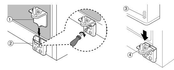
3) Insert the upper hinge shaft (⑤) into the hole (⑥). After levelling between the upper hinge hole (⑦) and the hole of the cabinet (⑧). Reattach hinge screws (⑨) and gound screw (⑩) in the clockwise direction.
