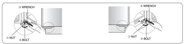
2) Please adjust the height difference between the doors by turning the bolt (②) clockwise ( ) or counter clockwise ( ).
