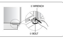
3) After adjusting the doors, the nut (①) turn clockwise ( ) until it reaches the lower end of the bolt, then tighten the bolt again with the wrench (③) to fix the nut(①).
