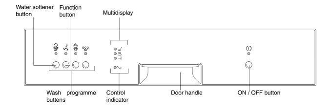
Water softener and function button: In addition to the indicated wash programme, the dishwasher water softener can be set using a combination of these buttons.
