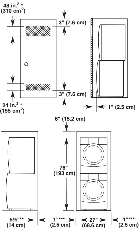
\*Min. top and bottom air openings for closet door.
