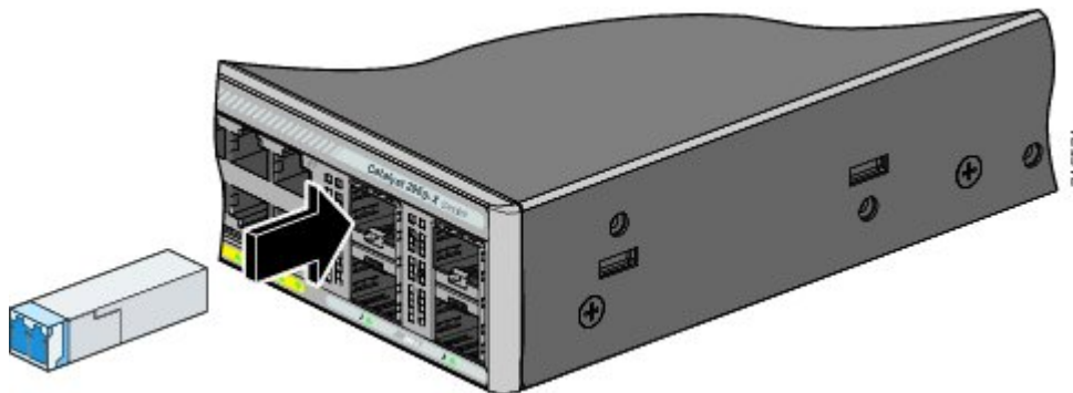
Figure 23: Installing an SFP Module
