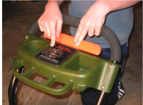
Figure 12. Moving backwards, the Direction Toggle set to Reverse and the Reverse Safety Button pressed down.
