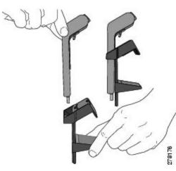
Step 5 With your phone idle (no calls), attach the USB cable to the USB connector on the bottom of the camera.Step 6 Adjust the mounting clip as needed to rest securely on your computer monitor.
