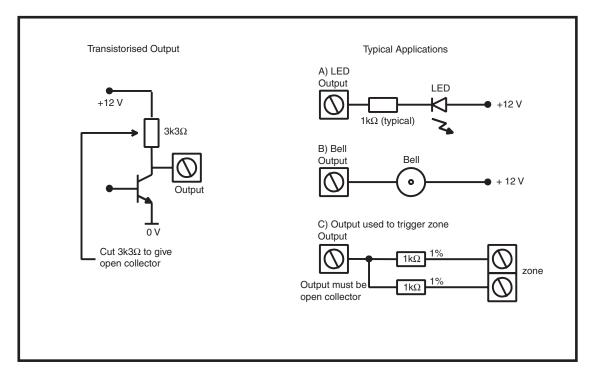
Figure 2-16. Output Configuration and Typical Applications
