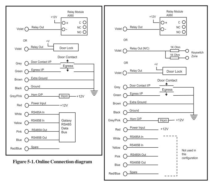
Figure 5-2. Standalone Connection diagram
