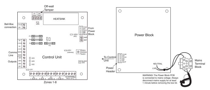
Figure 3-5. Power Supply Unit
