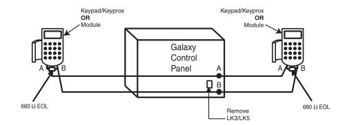
Figure 2-9. Twin AB Line Daisy-Chain configuration
