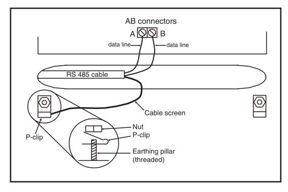
Figure 2-10. Connection of cable screen using P-Clip
