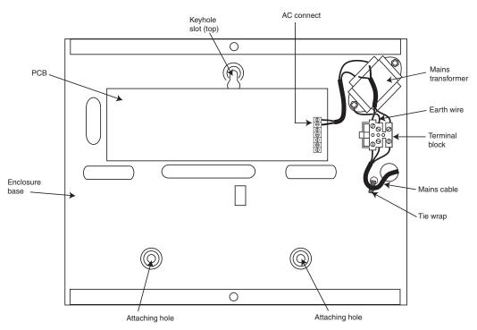
Figure 2-6. Securing the Mains Cable to the Enclosure Base
