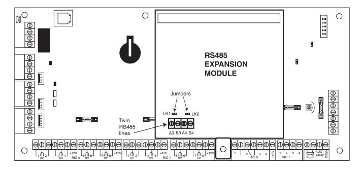
Figure 2-5. RS485 Expansion Module
