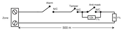
Figure 2-13. Preset 1 - End of Line Zone/Detector wiring
