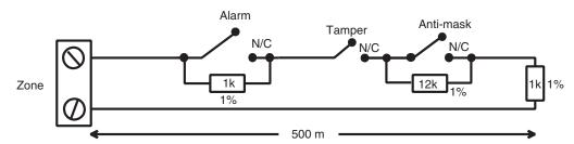
Figure 2-12. Preset 1 - Double balanced Zone/Detector wiring
