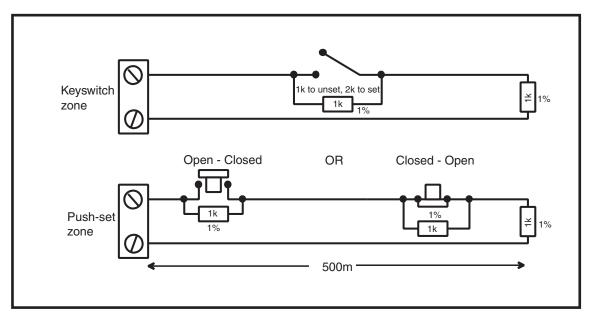
Figure 2-15. Terminator and Keyswitch Zone Wiring
