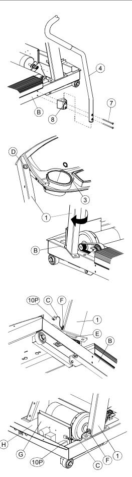
10. Locate the HANDRAIL CROSSBAR (#9). With the bend facing upward and pitched toward the DISPLAY CONSOLE, carefully place the HANDRAIL CROSSBAR between the user LEFT AND RIGHT HANDRAILS (#4) as shown and align the mounting holes. Insert one SHORT MOUNTING BOLT (#6) on either end of the HANDRAIL CROSSBAR and tighten using a 5/32" hex key wrench.
