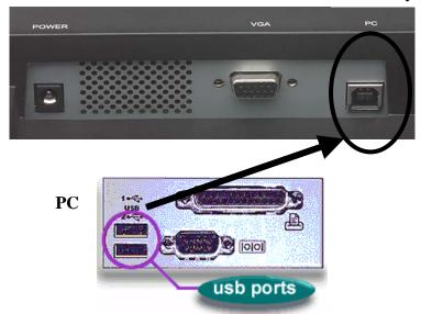
Figure 7 – Connecting a PC to MemoryFrame
