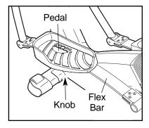
pedals forward or backward to the desired position, and retighten the knobs. Make sure that both pedals are in the same position.
