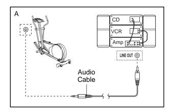
B. Plug one end of a 1/8" to RCA stereo audio cable (available at electronics stores) into the jack beneath the console. Plug the other end of the cable into an RCA Y-adapter (available at electronics stores). Next, remove the wire that is currently plugged into the LINE OUT jack on your stereo and plug the wire into the unused side of the RCA Y-adapter. Plug the RCA Y-adapter into the LINE OUT jack on your stereo.
