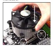
Turn over the mainboard to confirm that the clip-ends are correctly inserted.
