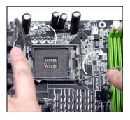
After confirming the CPU direction for correct mating, put down the CPU in the socket housing frame.
