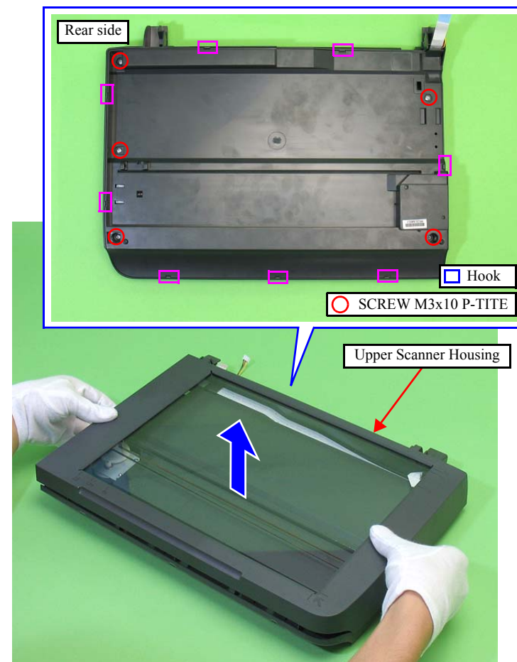
Figure 4-106. Removing the Upper Scanner Housing
