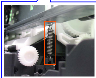
Figure 4-71. Removing the Main Frame (1)
