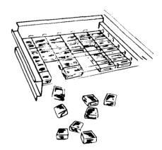
5. Cubes fall into the storage bin. When the bin is full the ice maker shuts off automatically and restarts when more ice is needed.
