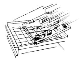
2. When the desired thickness is reached, the ice sheet is released and slides on to a cutter grid. The grid divides the sheet into individual cubes.
