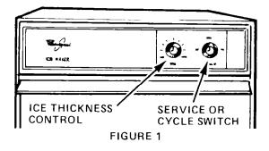
2. To start the normal ice making cycle, turn service or cycle switch to "ON."
