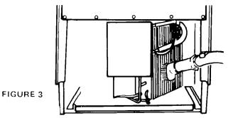
**4**. Remove dirt and lint from the condenser fins with a soft brush and then use a vacuum cleaner to remove the dirt from the unit compartment (Figure 3).
