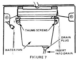
**2.** Remove the water pan by unscrewing the two thumb screws (Figure  $7^{1}$ .
