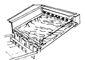
1. Water is constantly circulated over a freezing plate. As the water freezes into ice the minerals in the water are rejected. This produces a clear sheet of ice with a low mineral content.
