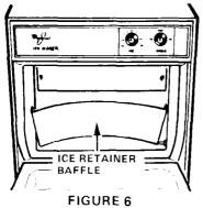
1. Remove ice retainer baffle by flexing it (Figure 6) and then slide it off the studs.
