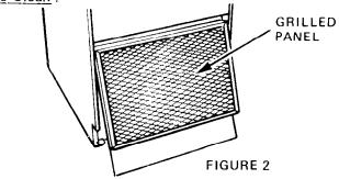
1. Disconnect electrical power supply to the machine or place the service switch in the "OFF" position. The condenser fan should not operate while removing dirt from the condenser.
