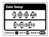
Set the Date and Time as desired by pressing the **RIGHT** and **LEFT** direction control buttons to choose the specific setting and the **UP** and **DOWN** buttons to change each setting.
