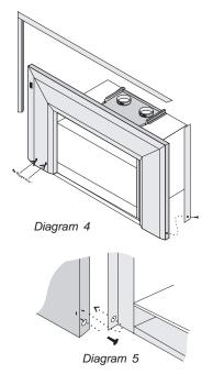
11) Push the Regency logo plate into the two holes in the bottom left corner of the faceplate.
