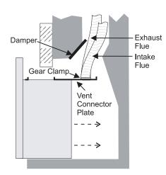
Connect the 2nd liner to the exhaust collar marked with an "E", seal connection with high temperature silicone. Secure with gear clamp.
