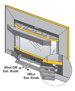
Slide the Robert Shaw valve extension knobs onto the valve knobs. Match the correct ext, knob with the valve knob.
