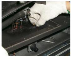
Note: when installing the burner assembly be sure to slide the aeration adjustment wire through the hole in the base of the burner tray.
