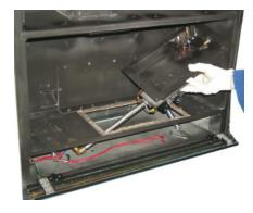
10) Remove the valve by removing the 3 screws in the base of the valve tray.
