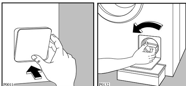
Unscrew and remove the filter.
