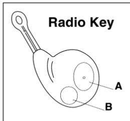
The Radio Keys are powered by a long life 3v Lithium battery (type CR2032 or equivalent). With normal usage a new battery should last between 3 and 5 years. Replacement batteries can be obtained from your Cobra Dealer.
