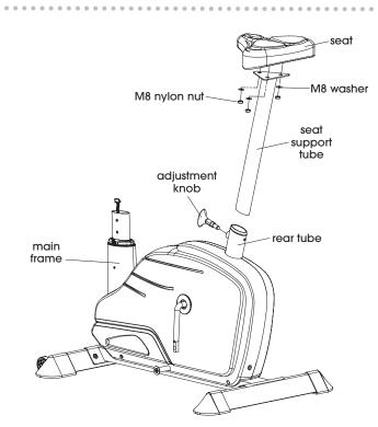
Figure 2 - Install Seat to Main Frame
