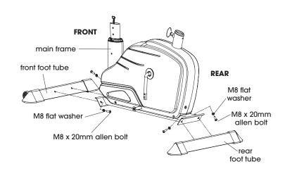
Figure 1 - Install Foot Tubes to Main Frame
