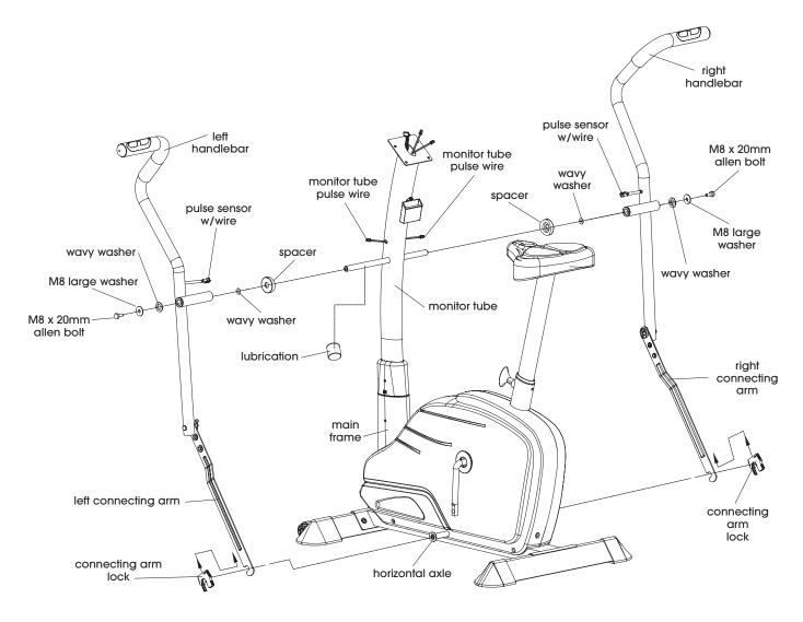
Figure 4 - Install Handlebar Assembly
