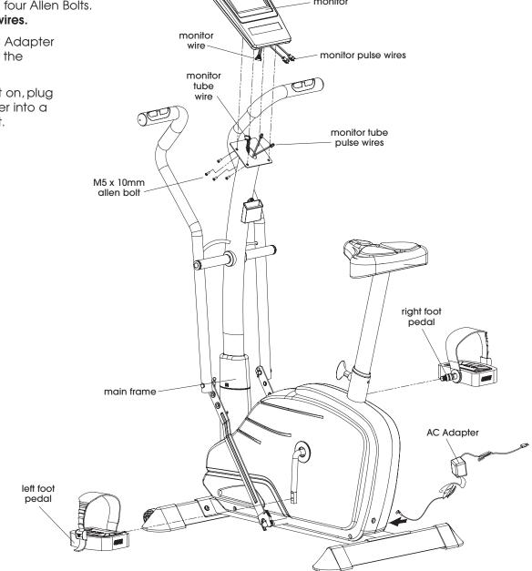
Figure 5 - Install Foot Pedals, Monitor and AC Adapter
