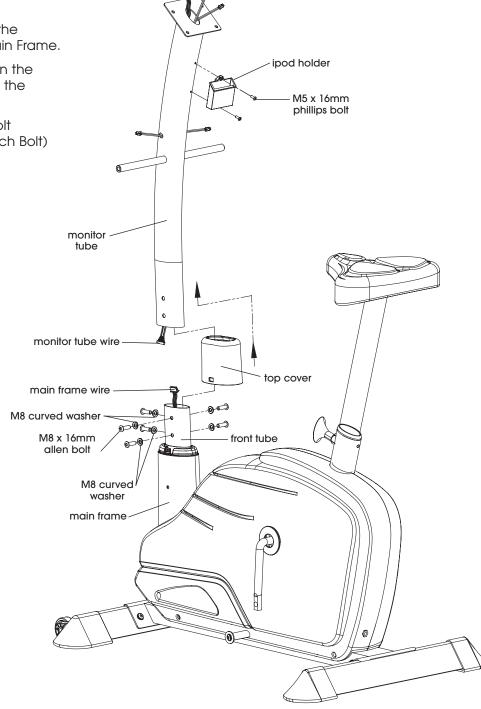
Figure 3 - Installing Monitor Tube
