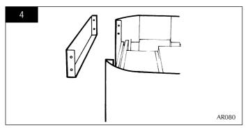
3.8 Locate the lower panels onto the lugs as shown. See diagram 5.
