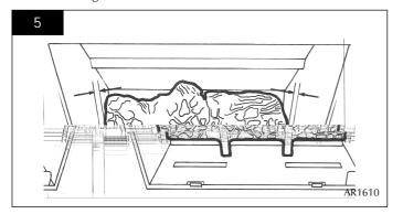
7.2 Place log B on the left-hand side of the burner with the location bar on the underside of the log fully located in the long slot of the burner. Make sure the log is as far to the left as possible. See diagram 6.
