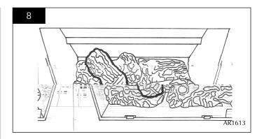
7.5 There are two ash panels which lay across the front of the burner skin. Place the panel with the flat edge facing the left side of the firebox. There are location holes on this log which fit over the screw holes of the burner skin.
