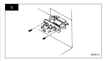
3.5 To remove the pilot injector, undo the compression nut on the pilot feed pipe and withdraw the injector which will be hooked onto the olive. When replacing an injector always make sure it is hooked onto the olive before inserting it into
