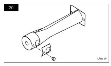
10.5 Reassemble in reverse order with correct aeration plate(s).
