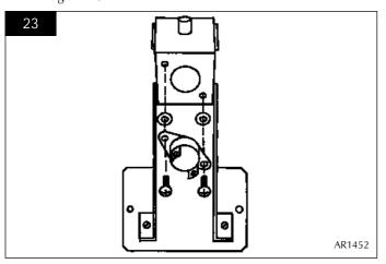
9.6 Feed the cable back through the hole as you replace the bracket. When the bracket is located correctly it will sit flush with the back panel without force required. If not positioned correctly the bracket will sit at an angle. See Diagram 24.
