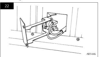
9.5 Refit the new sensor, ensuring that the plastic spacers are between the sensor and the bracket. Refit the leads. See Diagram 23.
