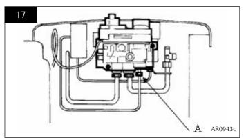
7.3 Reassemble the interrupter block and leads. Secure the thermocouple connection in the rear of the gas control (Do not overtighten). Turn the gas supply on and check the entire pipework and valve joints for any leaks.
