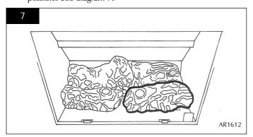
7.4 Place log D across from the rear log A to log B on the left-hand side. There are cut-outs in both logs for location. See diagram 8.
