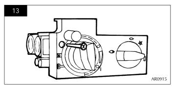
4.3 To release the right-hand side of the control cover insert the narrow blade screwdriver into the slot shown in diagram 14. Lever it gently and pull from the right-hand side at the same time. The cover will now come off. There is a small cylindrical metal spacer inside the cover; this must be kept and replaced on the fixing screw during reassembly.
