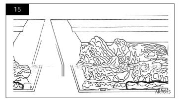
5.7 Place log E across from the rear of log A to log C on the right-hand side. Again, there are cut-outs for location. The front of the log should sit on the front ash panels and should fit tight to log C. See diagram 16.
