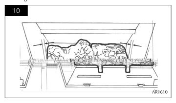
5.2 Place log B on the left-hand side of the burner with the location bar on the underside of the log fully located in the long slot of the burner. Make sure the log is as far to the left as possible. See diagram 11.
