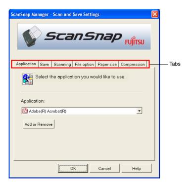
You can configure the save and scanning settings of the ScanSnap with the six tabs.
