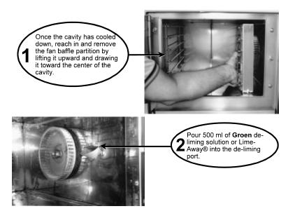
The process for de-liming your HY-6E (CE) Steamer is simple, tool-less and quick.
